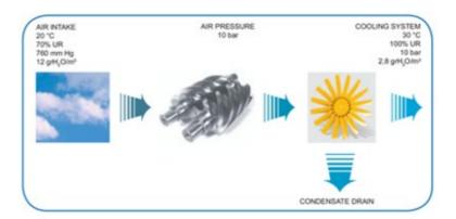
Compressed air is cooled at 30°C and condensed water vapour is separated, while 2.8 gr of water for every Nm³ of air that condense can remain in the air (compressed at 10 bar as in the example) in vapour form.
